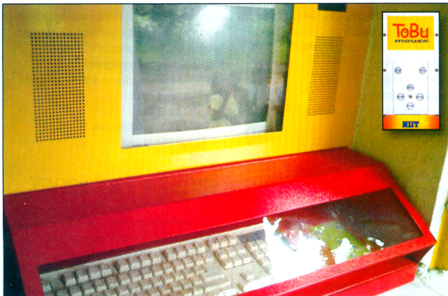
A typical Hole in the Wall computer kiosk and (inset) the touch-sensitive mouse.
